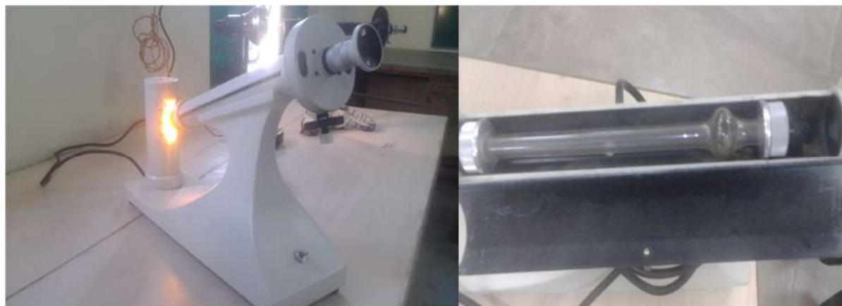
Figure 1: Left-panel: Polarimeter instrument and its set-up. Right-panel: Place of the solution tube in the instrument
