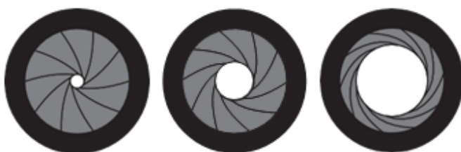
Fig.1.2 Iris diaphragm showing different aperture sizes
