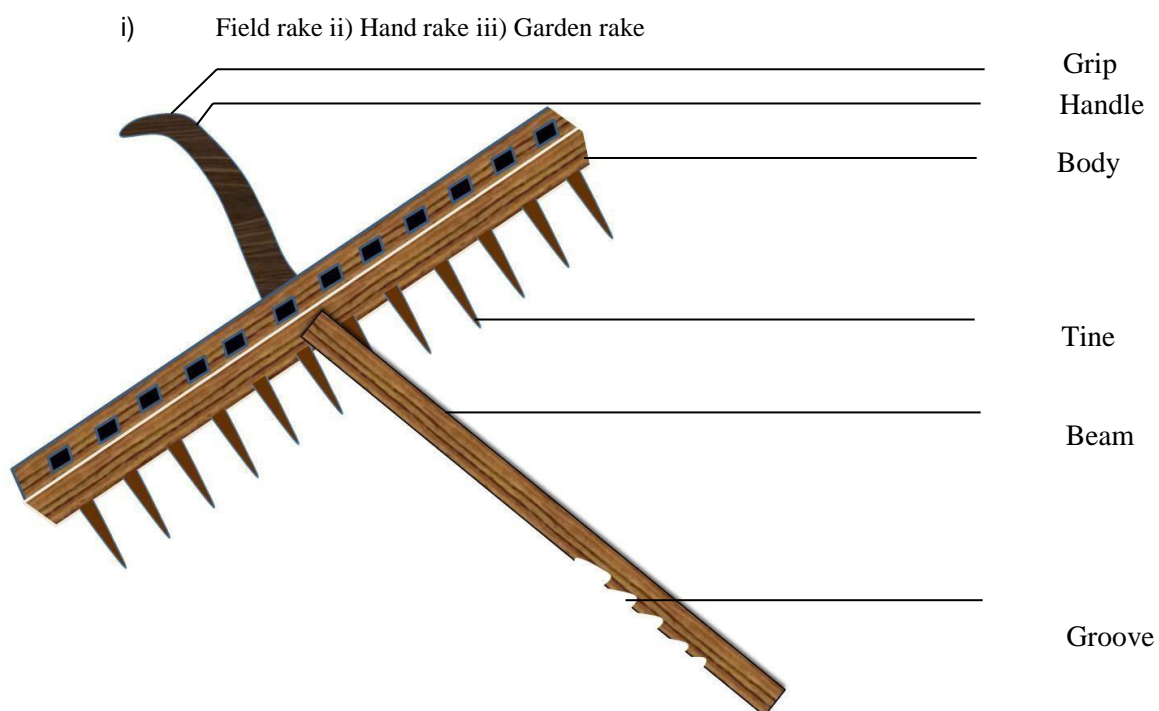
Fig. Field rake and its different part
