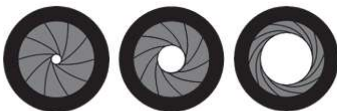
Fig.1.2 Iris diaphragm showing different aperture sizes
