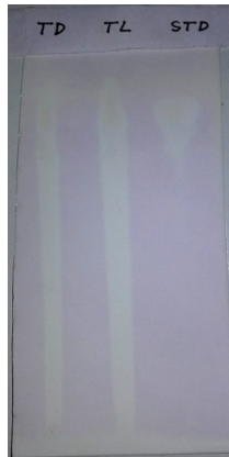
Figure 1: Thin layer chromatography antioxidant activity analysis of Black tea water extracts and Ascorbic acid. TD- Tea Dust, TL- Tea Leaf, STD- Ascorbic acid
